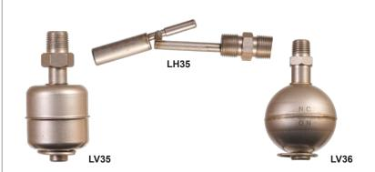
Offered in both vertical and horizontal configurations, the general purpose high-temp float level switches provide reliable liquid level detection of relatively clean water, diluted chemicals and light weight oils with a 30VA or 100VA reed switch output. Media examples include hot deionized water and cooking oil. The stainless steel liquid level sensors are mounted vertically inside the tank or horizontally through the tank wall as a high level alarm or low level alarm.
